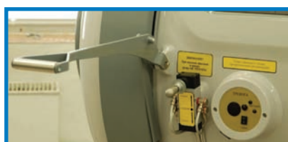
Control handle for the bayonet lock is for emergency use only when there is no pressure in power circuit
